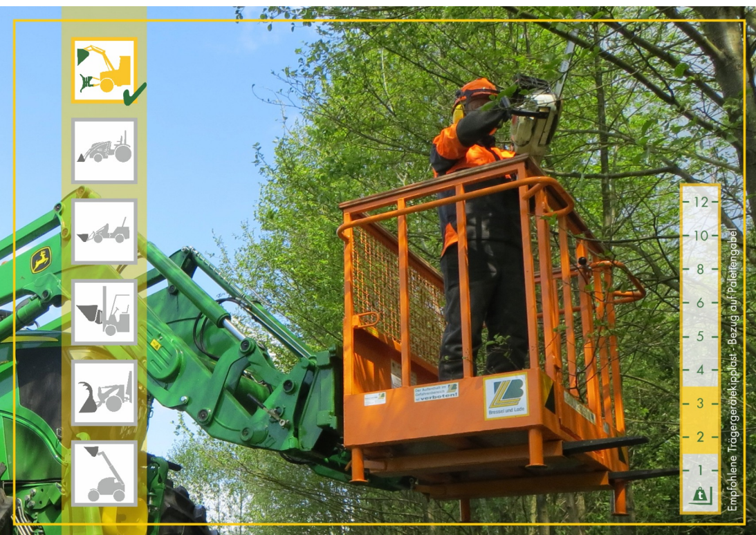
Working platform manufactured according rules of the german "LSV-Information T01"
