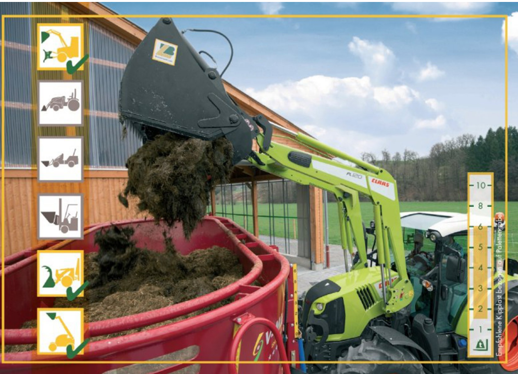
The Silagecutter is designed for clean cut of all kinds of silage. The bendsave cutting shield cuts even extrem compressed silage.
