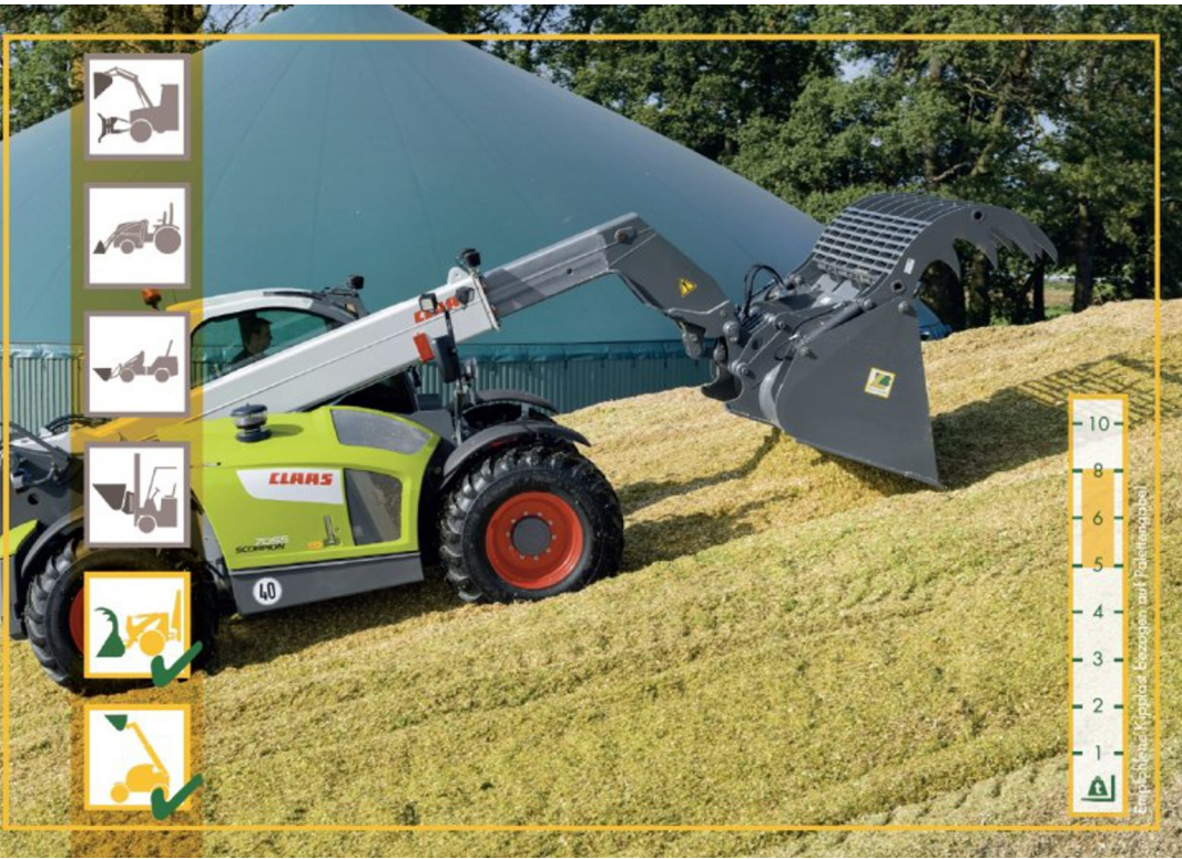
The Silagebucket is designed for collection and transportation of silage and loading of manure.
