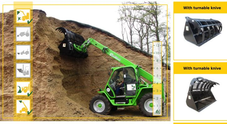
The Silagebucket is designed for collection and transportation of silage and loading of manure.
