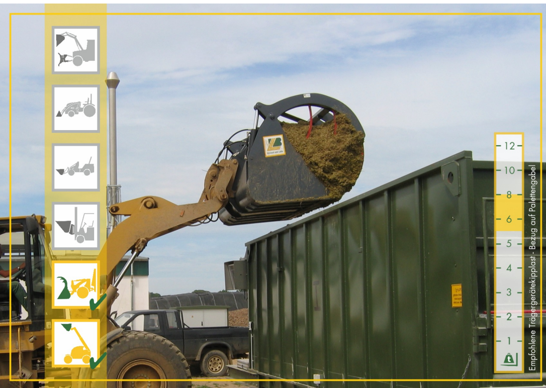
The Silagebucket is designed for collection and transportation of chopped silage.
