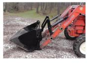
This rebuilt Kit allows to refit old auto-latch front loaders to the Euro-System with tipping function.
