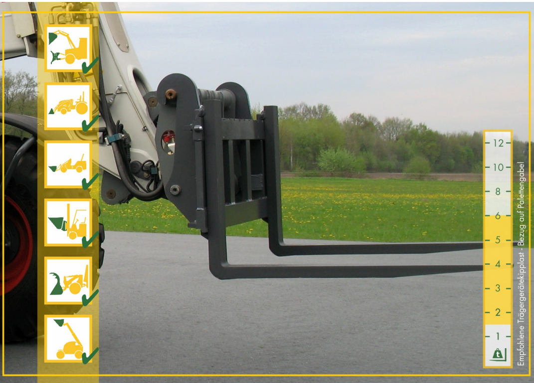
The pallet fork is designed for loading goods on pallets. The high value pallet fork tines are adjustable in the distance to each other.
