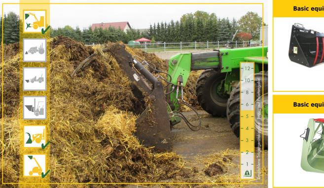
The Manure Bucket is heavy duty designed for loading manure. By removing the screwed sideparts it is easier to load heavy manure.
