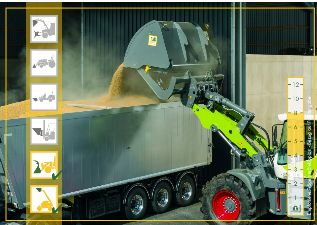
A High tip bucket raises the unload height and the dumping angle.
