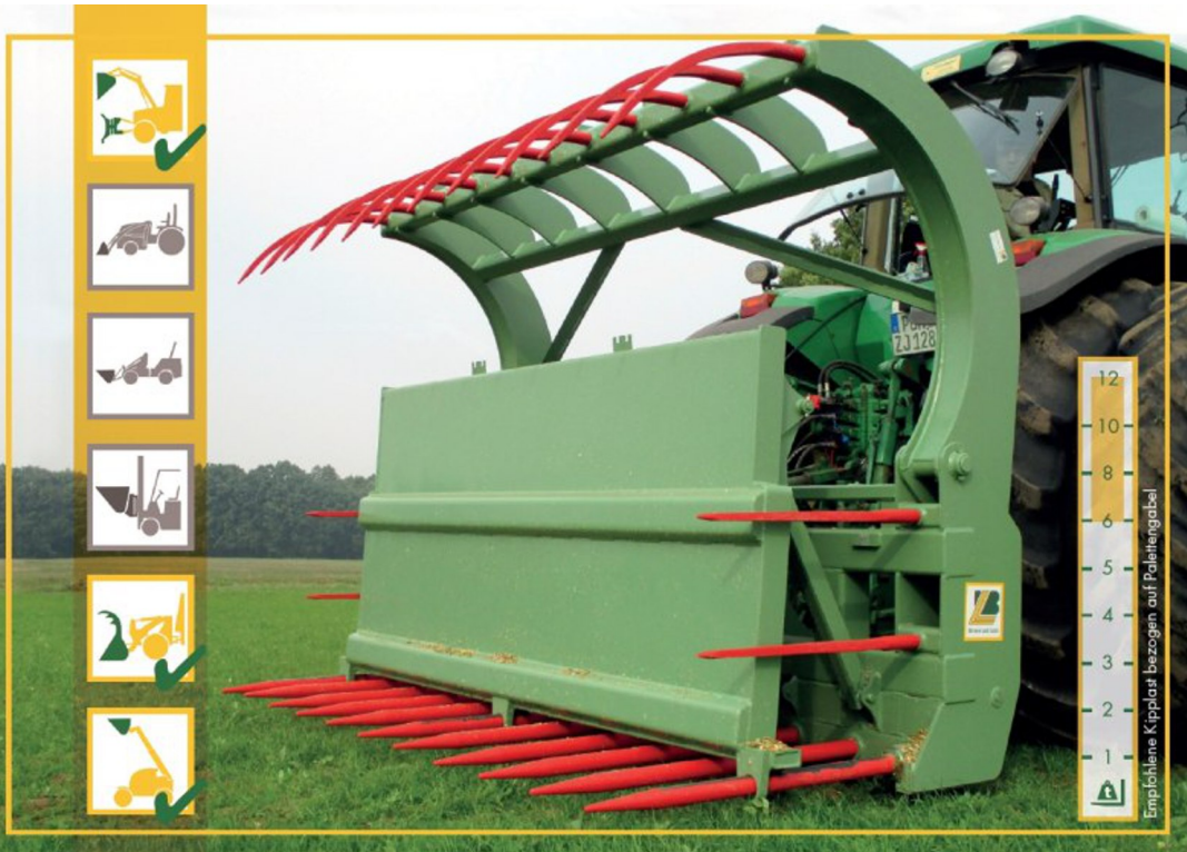
The Green forage grapple is an attachment for pushing silage with heavy loaders.
