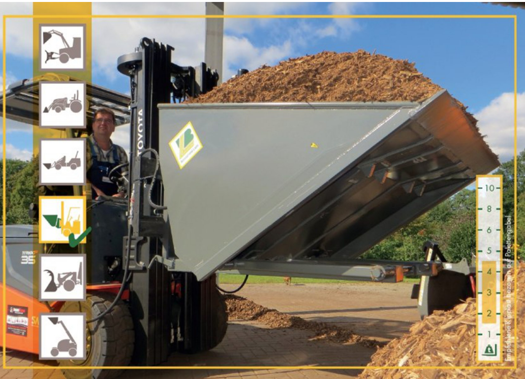
This bucket can be connected quickly on the pallet forks.
