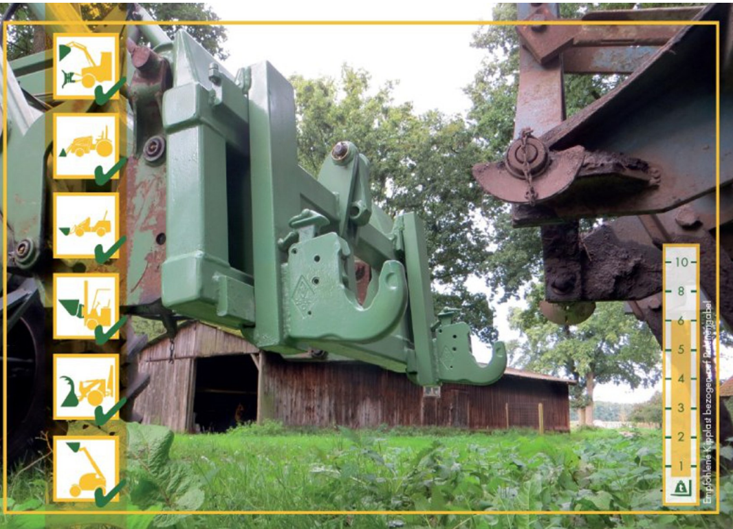
Attachments with 3-point linkage or municipal quick coupling plate can be picked up with this adapterframe.
