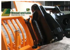
Adapter for MF telehandler to Euro-quick-coupling system
