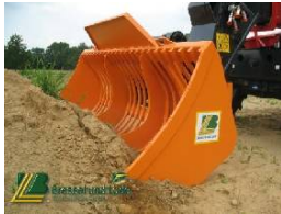
Model with rollback protection connected to a MF telehandler mit adapter frame (pic. 646)
